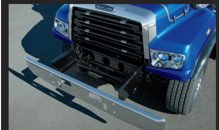
Tilt hood with radiator-mounted stationary grille and front frame extensions.
